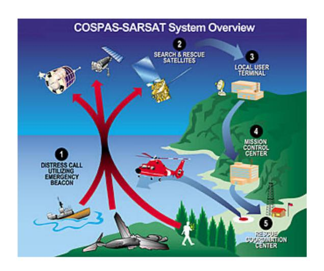
Small portable devices using the global COSPAS-SARSAT Satellite System and sending signals on the 406MHz frequency
